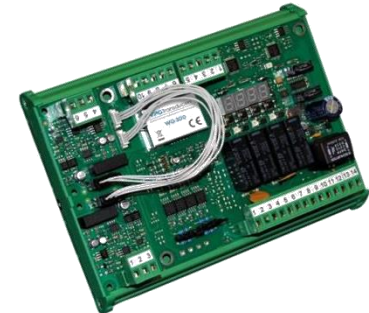
WG3 – safeguard to prevent overload of weighing machines.
